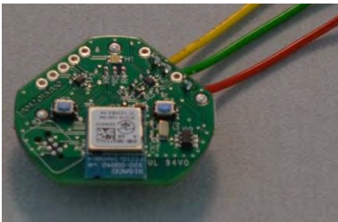
Figure 19: smartdoor Bluetooth module connections
