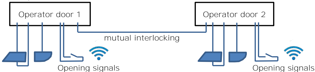
Figure 30: Principle-scheme double door airlock
