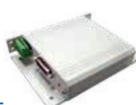
LAA-5 Single-axis PWM Amplifier 24-48VDC 3 Arms cont., 6 Arms peak +/- 10 Volt command input Single-axis PWM Amplifier
