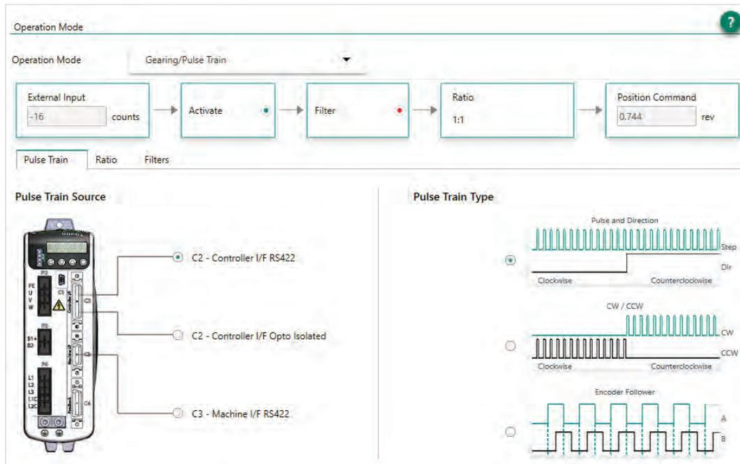
Figure 22-6. ServoStudio 2 – Motion Screen – Gearing/Pulse Train Mode
