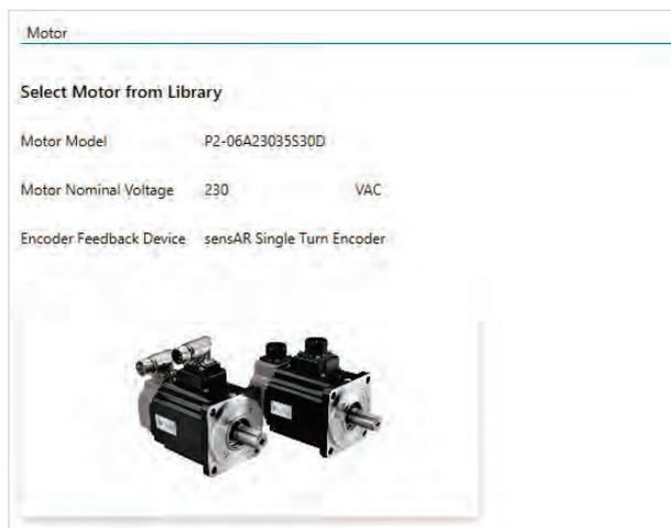
Figure 10-1. ServoStudio 2 – Motor Data from Electronic Motor Nameplate
