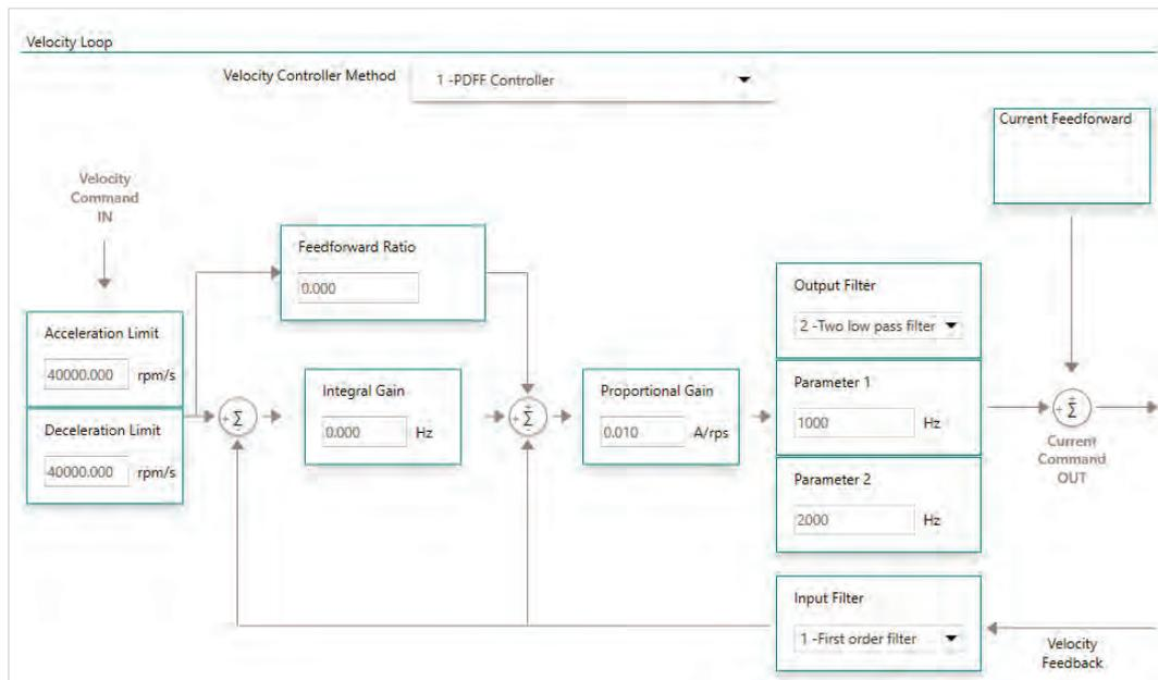
Figure 20-3. ServoStudio 2 – Velocity Control Loop – PDFF Controller
