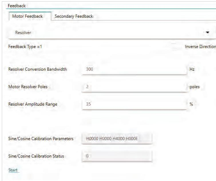
Figure 11-3. ServoStudio 2 – Feedback Screen – Example – Resolver
