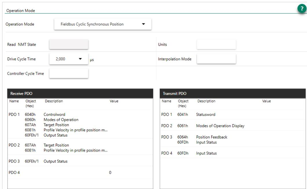
Figure 22-7. ServoStudio 2 – Operation Mode Screen – Fieldbus - Example
