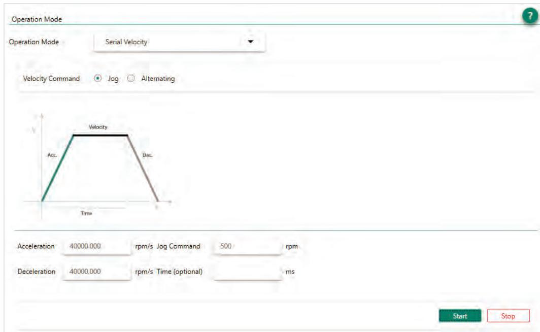
Figure 22-2. ServoStudio 2 – Motion Screen – Serial Velocity Mode
