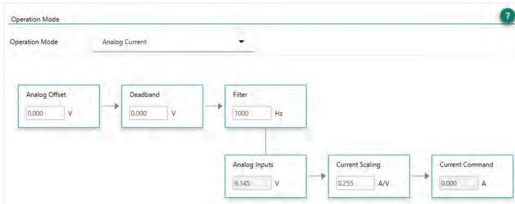
Figure 22-4. ServoStudio 2 – Motion Screen – Analog Current Mode
