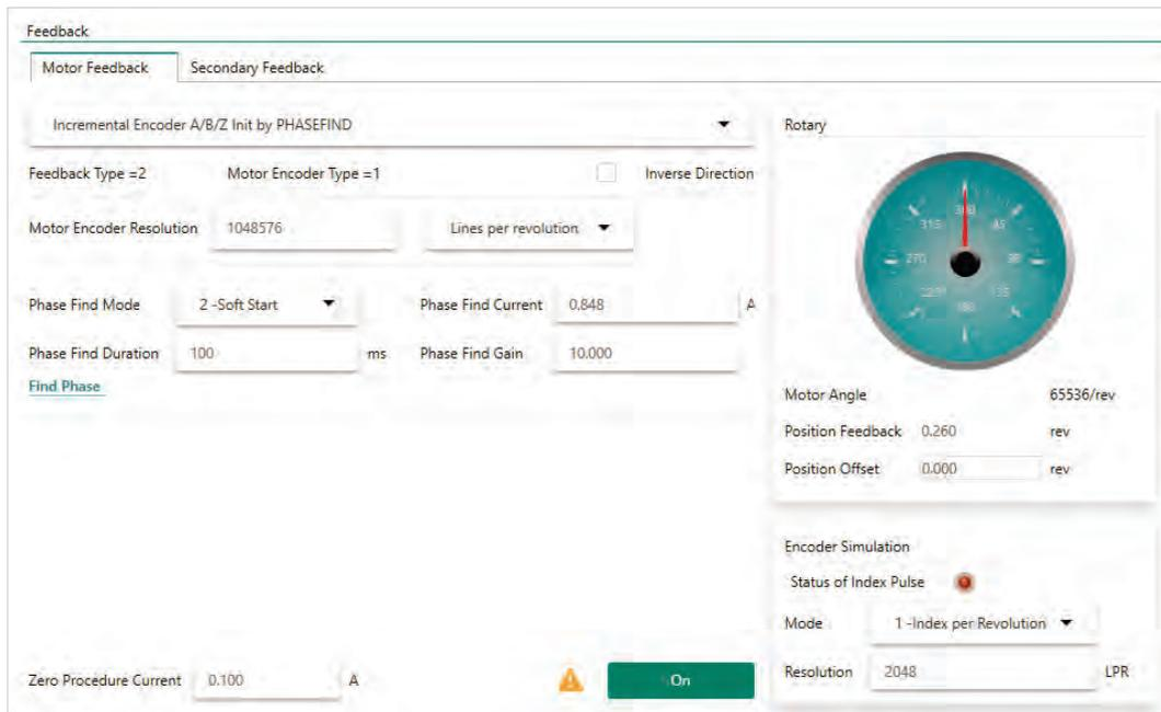
Figure 11-2. ServoStudio 2 – Feedback Screen – Example – Incremental Encoder
