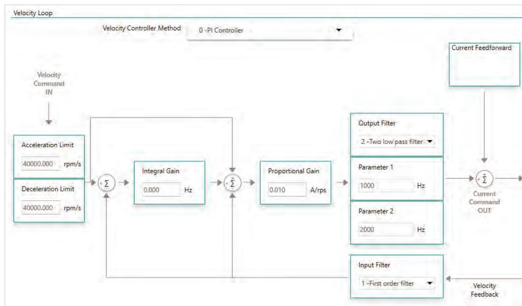
Figure 20-2. ServoStudio 2 – Velocity Control Loop – PI Controller
