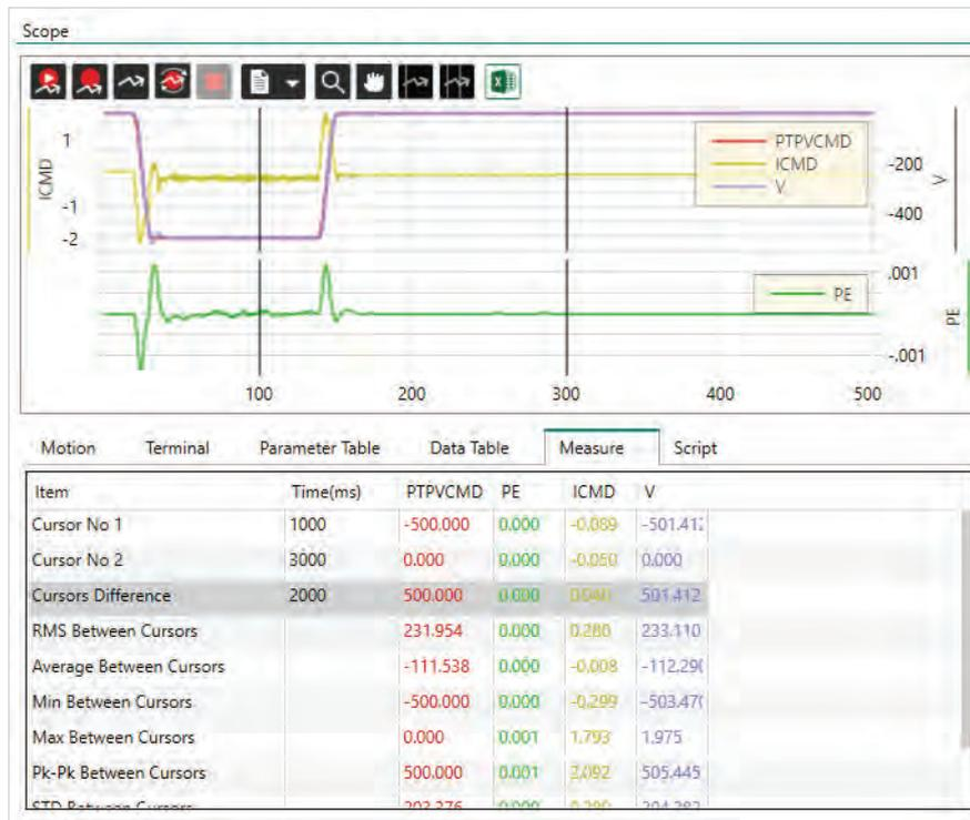
Figure 26-15. ServoStudio 2 – Scope Measurement Tab
