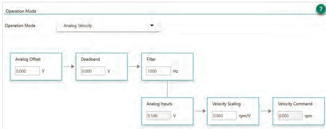
Figure 22-5. ServoStudio 2 – Motion Screen – Analog Velocity Mode
