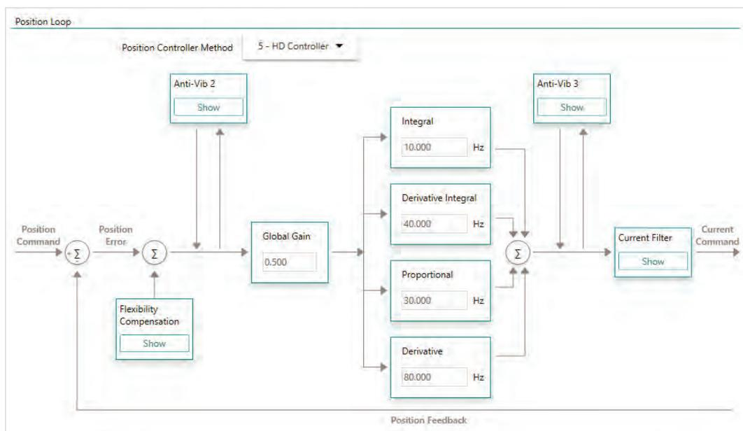
Figure 21-1. ServoStudio 2 – Position Loop – HD Controller Screen
