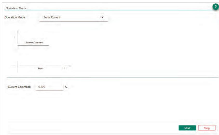
Figure 22-1. ServoStudio 2 – Motion Screen – Serial Current Mode
