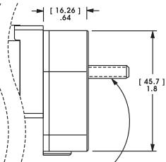
**Note:** Lead-screw extends beyond encoder on specific captive and non-captive motors. External linear shaft extension is available upon request.
