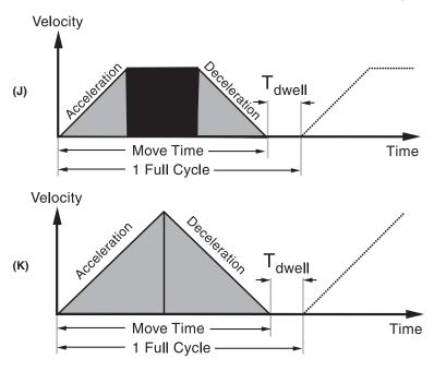
If using a **trapezoidal** (J) or **triangular** (K) move profile, the following is needed...
