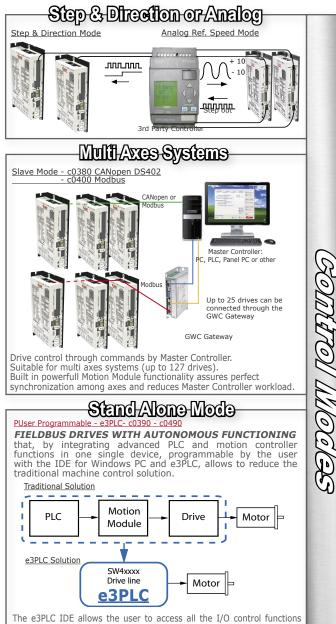
The e3PLC IDE allows the user to access all the I/O control functions and resources, provided by the drive, and to locally program its Motion Control Module, which can also be synchronized with other drives and events of the controlled process. Thanks to the advanced functionalities of the Power Motion Module, an integrated Real-time Process Module, applications can be easily created for special applications such as: • Labellina
