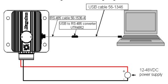
After wiring as shown, turn on power supply.
